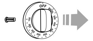
Loosen the locking screws inside the oven temperature control knob.
